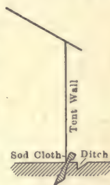
FIG. 192.—Sod-cloth and Ditch.
